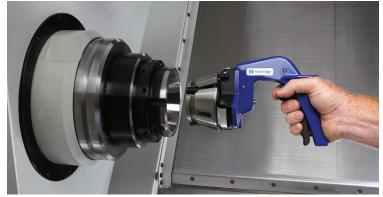
Hardinge FlexC<sup>™</sup> Low Profile Dead-Length<sup>®</sup> Collet System Style DL — 65mm
